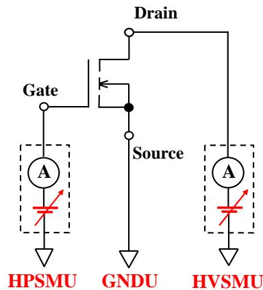
HPSMU can be used for the measurement up to 200 V. And HVSMU supports the high voltage measurement up to 3000 V.
