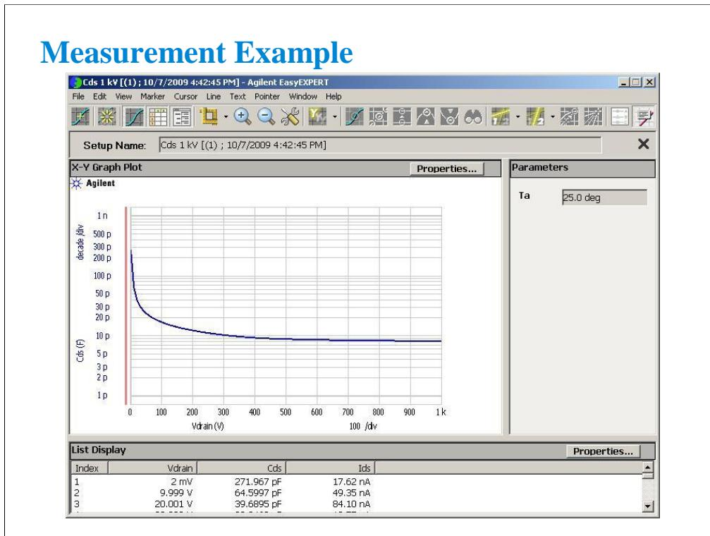
Perform measurement. The Data Display window will show the measurement result as shown in this example.
