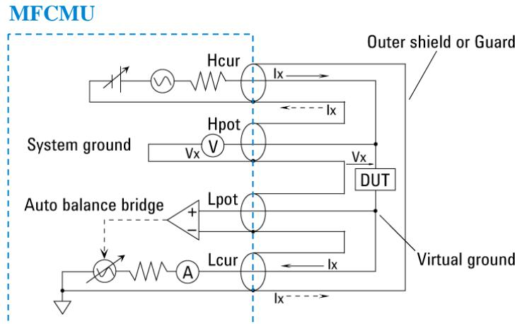
Generally, any mutual inductance, interference of the measurement signals, and unwanted residual factors in the connection method incidental to ordinary termination methods will have significant effects on the measurements, especially at a high frequency. The MFCMU employs the four-terminal pair (4TP) measurement configuration which permits easy, stable, and accurate measurements and avoids the measurement limitations inherent to such factors.
