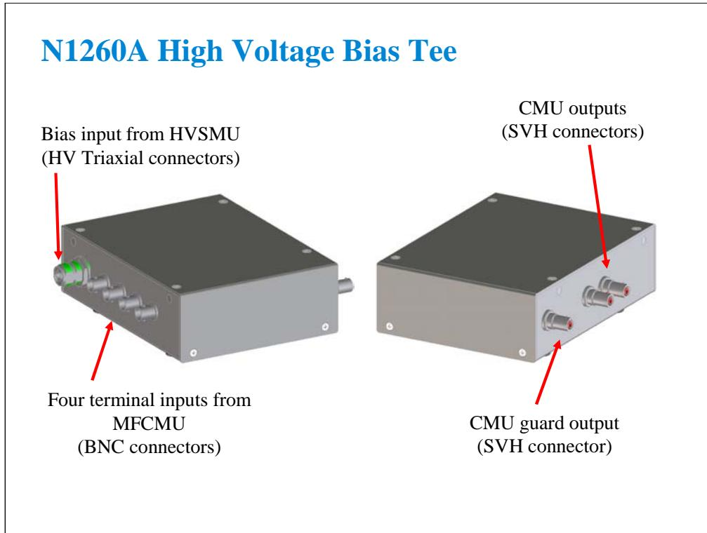
High voltage bias-T is used to perform the high voltage C-V measurement. The C-V measurement up to 3000 Vdc can be realized by using the bias-T, MFCMU, and HVSMU.
