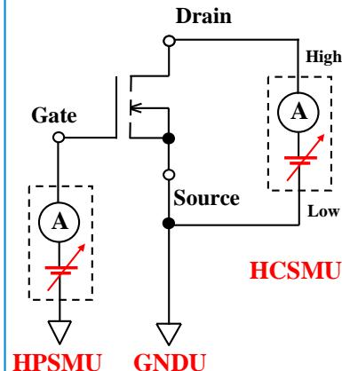
Before performing measurement, choose appropriate SMU type for connecting to the device terminal.
