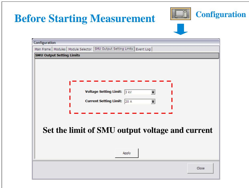
The HVSMU and HCSMU output can be limited by using the Configuration window SMU Output Setting Limits tab screen. This is effective for preventing the probe tip from burning out.
