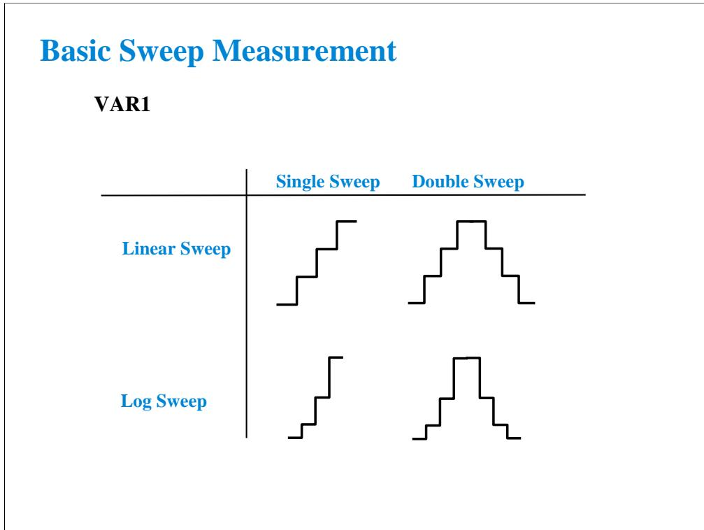
The SMUs can now sweep up to a value and then back down (double sweep). This feature is useful when the device must be tested without abruptly removing the forcing condition.
