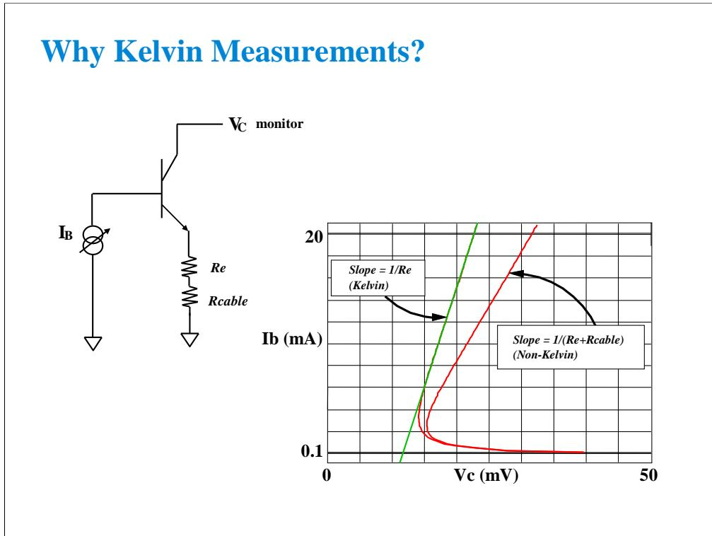
In the example above, the device is connected with a SMU on the base sweeping current, a voltmeter on the collector, and the emitter is grounded with a Kelvin SMU. The base SMU does not have to be Kelvin since we are only forcing current and do not care about measuring the cable loss in the base. Also, the collector SMU is being used only as a high impedance voltmeter, so there is no cable loss in this lead.
