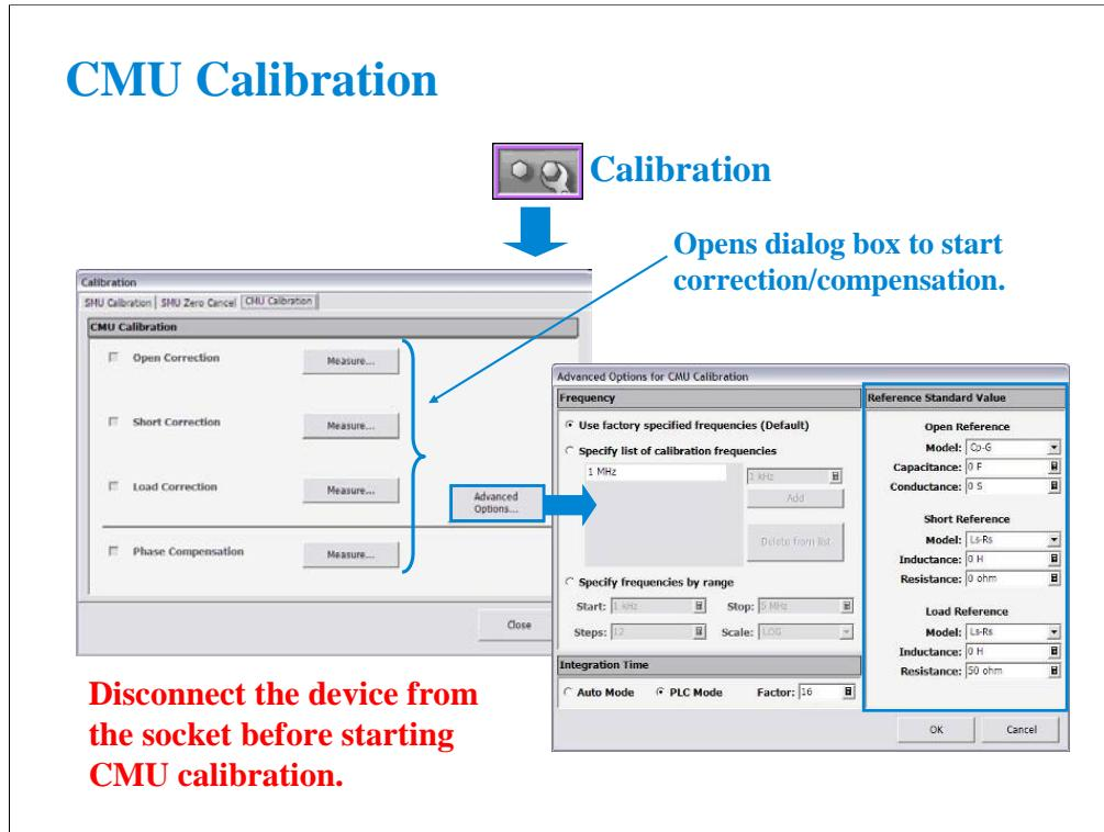
Open the Calibration window and click the CMU Calibration tab to perform the CMU calibration.
