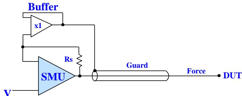
The guard connection is needed for the high voltage measurement and the measurement  $< 1 \text{ nA}$ . Below  $1 \text{ nA}$  a regular coax cable's capacitance dominates over the DUT (device under test) capacitance. What you see is cable charging current.  $I = C(dv/dt)$  where  $dv/dt$  is the rate of change of SMU voltage from one step to the next of a coax cable with no guard.  $C$  is the total capacitance of the cable.
