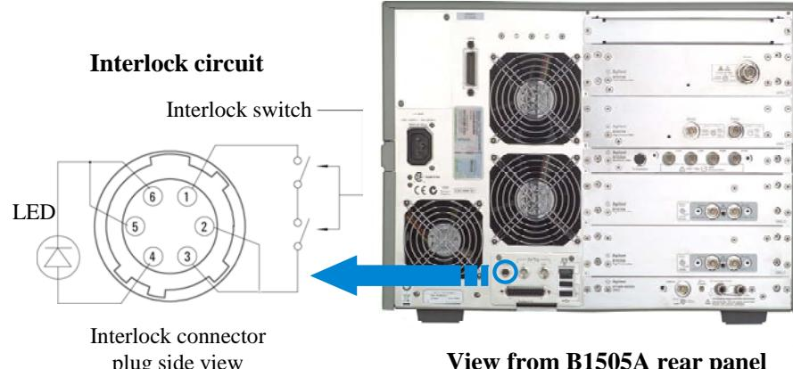
To prevent shock hazard, the B1505A will not operate above 42 V, unless you connect the interlock circuit.
