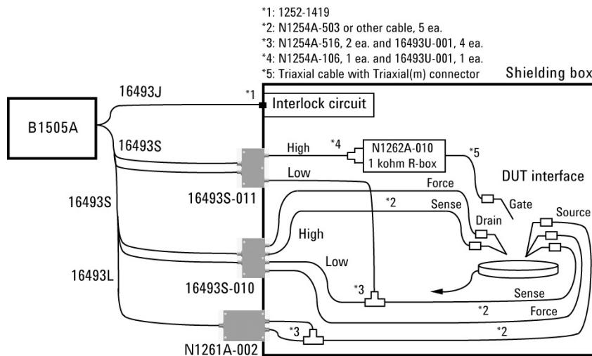
If the additional HCSMU is used for the measurement of the low current terminal such as MOSFET Gate, the 16493S-011 HCSMU Non-Kelvin adapter can be used instead of the 16493S-010 Kelvin adapter. The Non-Kelvin adapter converts the HCSMU connectors to two BNC connectors High and Low.
