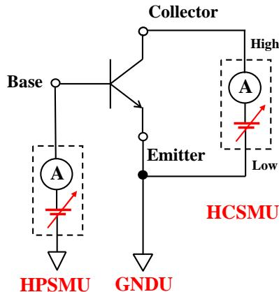
HPSMU can be used for the measurement up to 1 A. And HCSMU supports the high current measurement up to 20 A.
