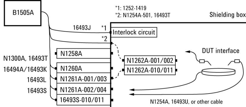
This is the image of measurement setup. The B1505A can be connected to several accessories as shown. The accessories can be connected to the B1505A directly by using the dedicated cables.
