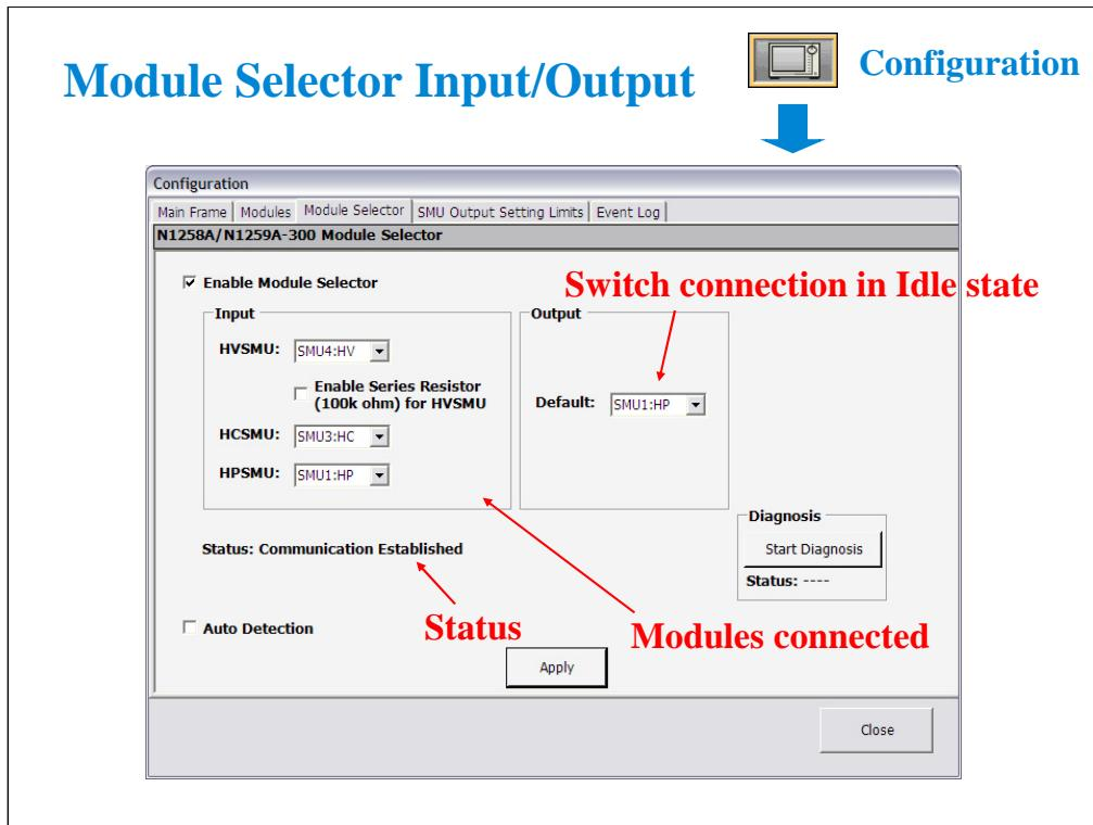
The Configuration window Module Selector tab screen is used to specify the input connections and the default setting of the module selector.
