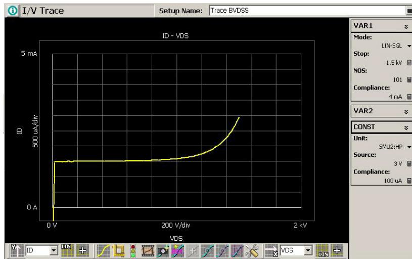
Perform measurement. The graph area will show the measurement result as shown in this example.
