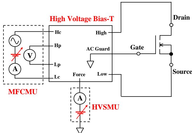
The above example shows the connections for measuring a power MOSFET Cds-Vds characteristics. MFCMU and HVSMU are connected to the high voltage bias-T as shown. And High, Low, and AC Guard are connected to Drain, Source, and Gate respectively.
