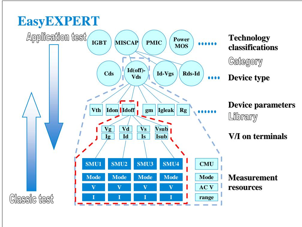
Instead of setting up the instrument hardware, the EasyEXPERT software focuses on the real task at hand for the engineer ---device characterization. All that you need to do is to connect the instrument to the device terminals as shown in the EasyEXPERT test parameters area.
