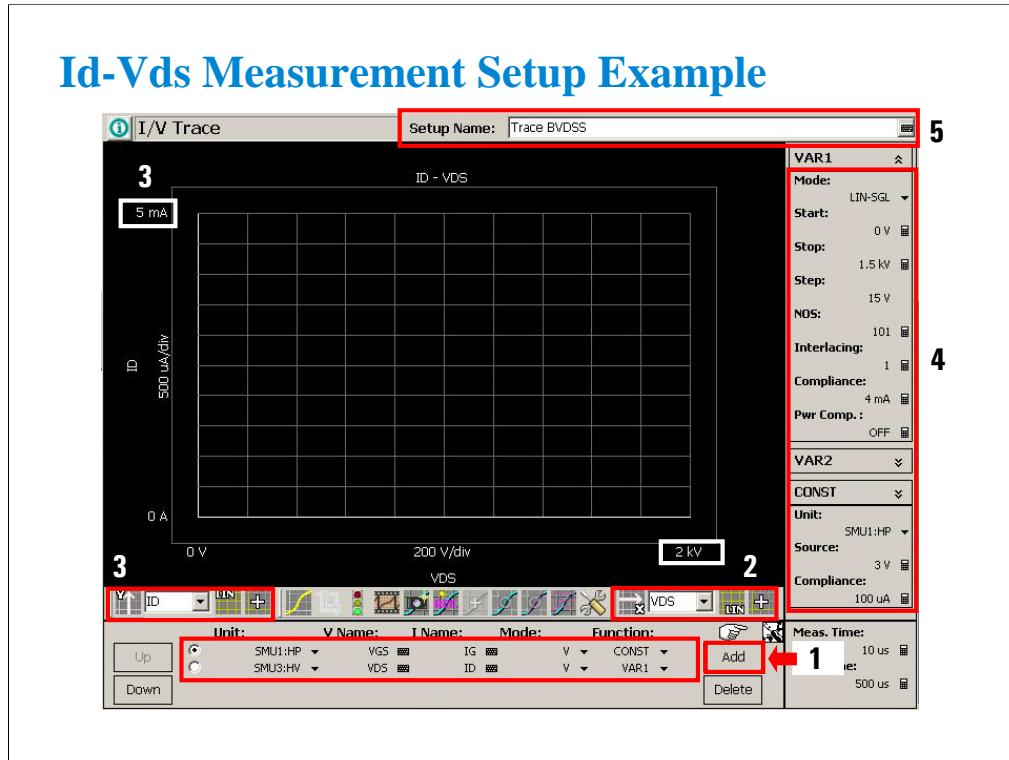
Display the Tracer Test screen and set the measurement condition.
