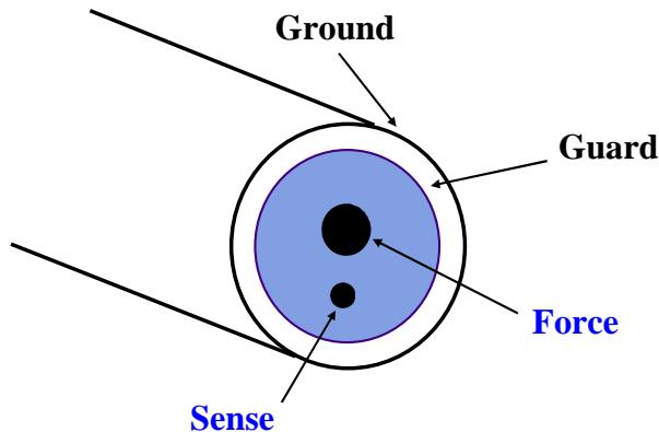
The triaxial cables are good for low current measurements. However, two cables are necessary for low resistance Kelvin measurements.
