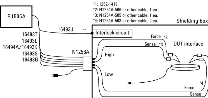
The module selector is used for the automatic switching of the measurement resources connected to DUT. The measurement resources are the HPSMU, HVSMU, HCSMU, and GNDU.
