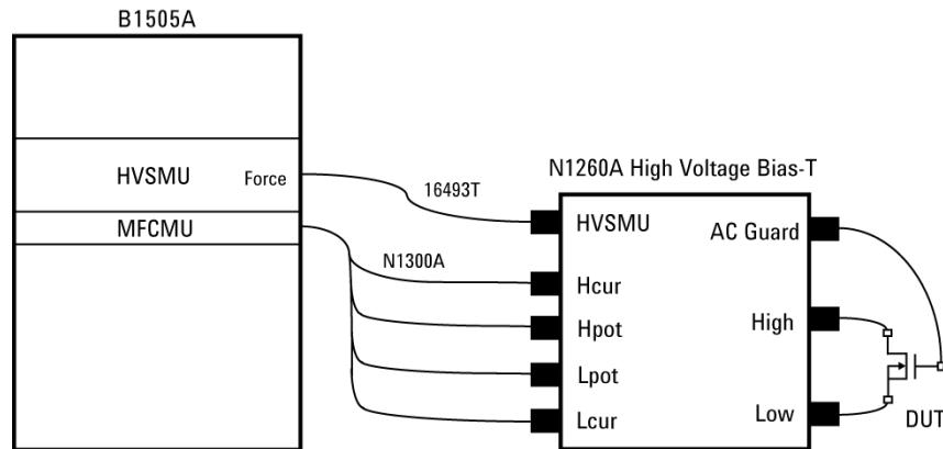
The high voltage bias-T is required for the up to 3000 V high voltage C-V measurement. The B1505A and DUT should be connected as shown.
