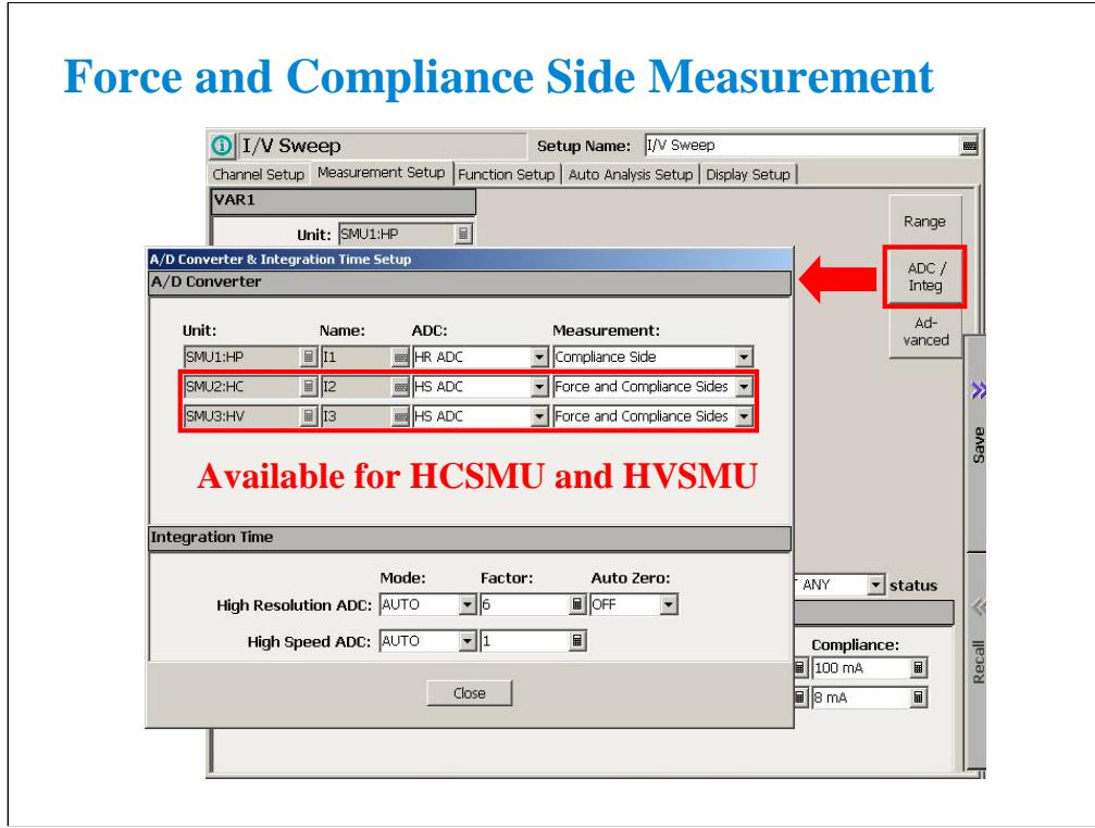
The HVSMU and HCSMU can perform the measurements for both force side and compliance side simultaneously. This means that the HVSMU/HCSMU can measure both voltage and current when it performs voltage or current output.
