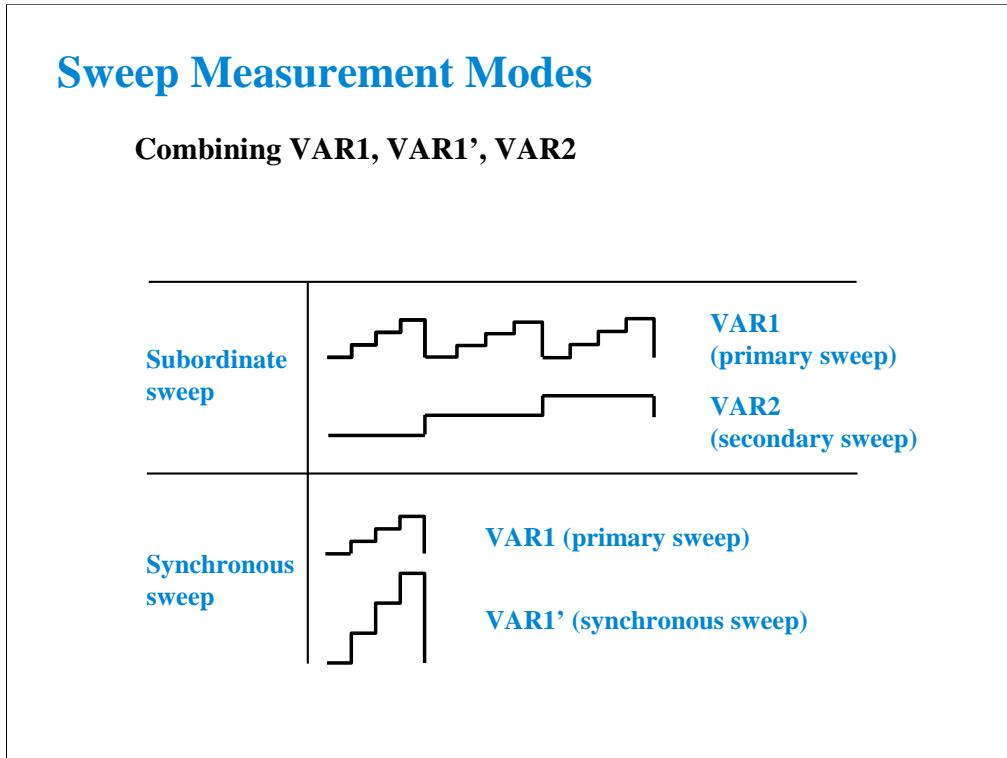
A subordinate sweep variable (VAR2) may be combined with the basic sweep variable (VAR1). This corresponds to the step knob and sweep knob of a curve tracer. This produces a family of curves. VAR2 may be called the secondary sweep.
