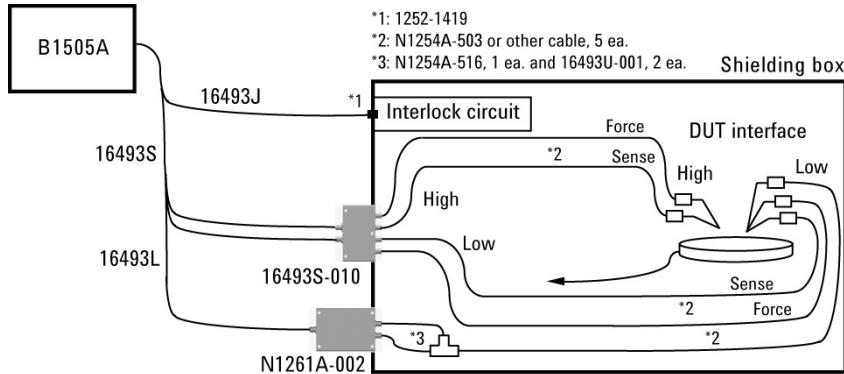
The 16493S-010 HCSMU Kelvin adapter converts the HCSMU connectors to four BNC connectors High Sense, High Force, Low Sense, and Low Force. This adapter must be used for the high current measurement to reduce the effect of the residual resistance.
