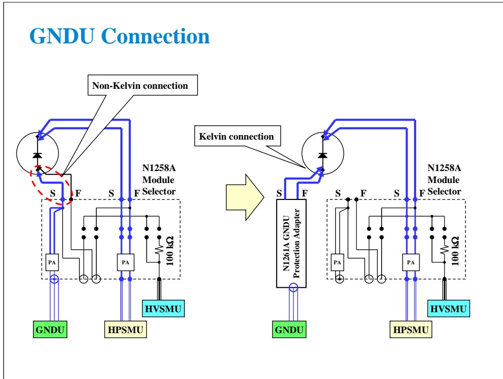
For the measurement using the module selector, the GNDU can be connected to the module selector GNDU input. This connection is especially effective for the measurement using the HCSMU because it makes cabling easy although it ends the Kelvin connection of GNDU in the module selector. This is no problem for the measurement with the HCSMU as no current flows to the GNDU.
