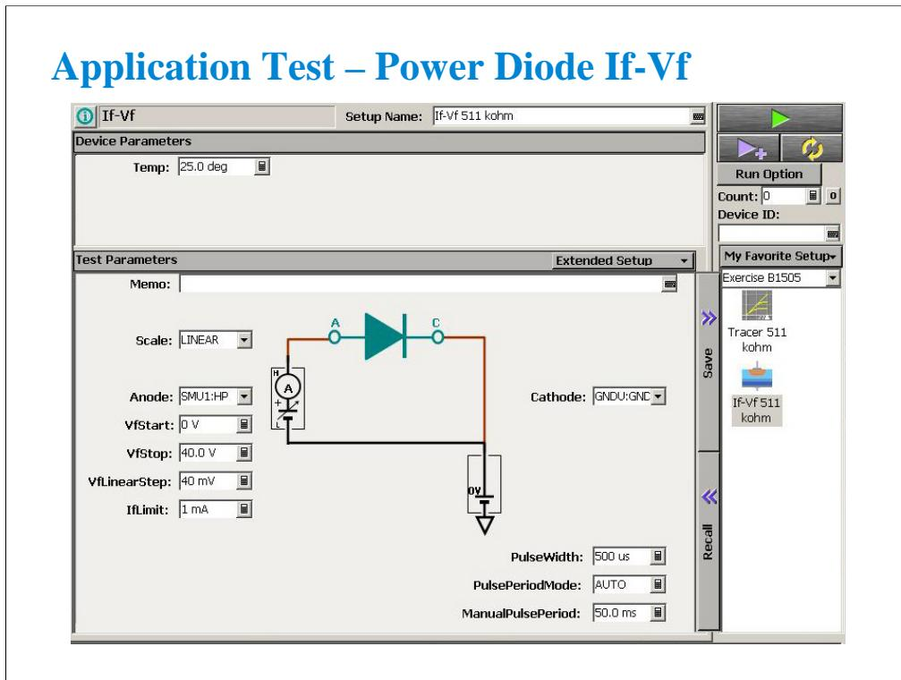
Open If-Vf application test in the Power Diode category. This test can be used for resistance measurement.
