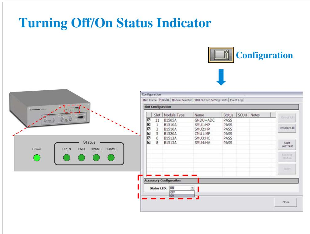
To make complete dark condition in the prober shielding box, the status indicator must be OFF.
