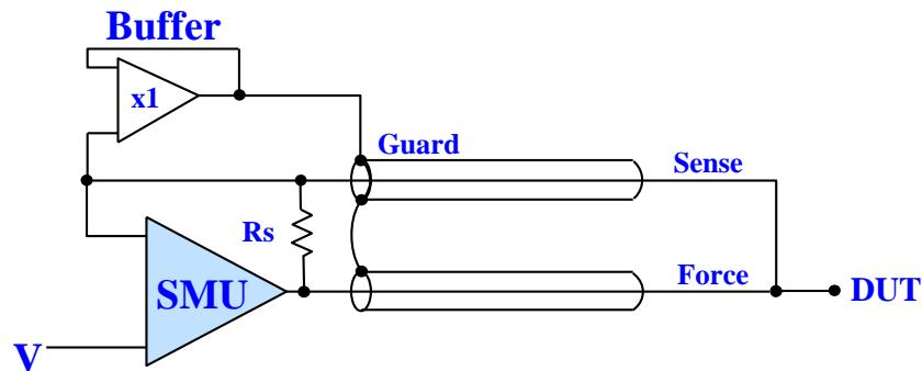
With the Kelvin connection, sensing is done at the DUT, eliminating the fraction of an ohm of cable resistance. The internal sensing resistor  $R_s$  is the only feedback path without the Kelvin connection.
